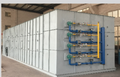
Hot-dip Galvanizing Furnace
